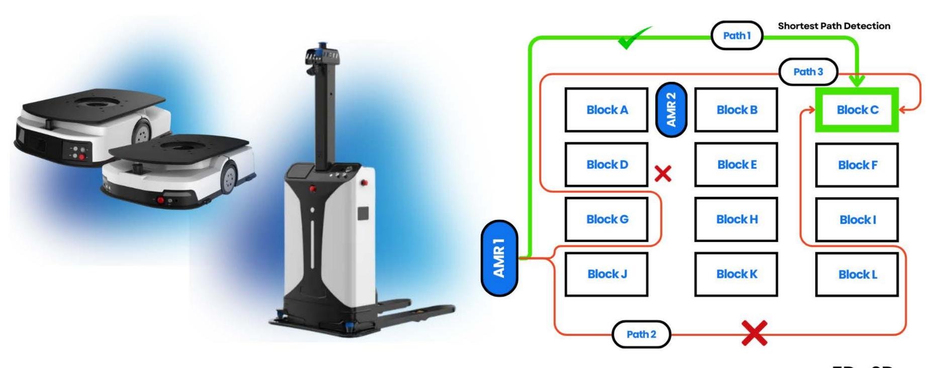
300 - 9000 KG Rated Load Weight 360 Obstacle Avoidance 8-9 Hrs Operating Time 10 mm Positioning Accuracy 1.3 - 1.7 m/s Rated Load Speed 3D - 2D Camera & Laser Obstacle Avoidance
